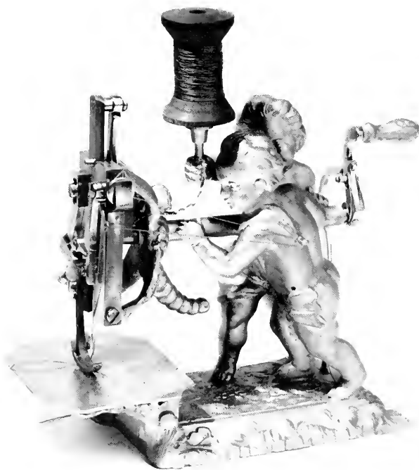
Figure 41.—THE CHERUB sewing machine was another Robertson first which was adopted by Clark. Robertson's patent of October 20, 1857, once again makes no claim for the design; neither does Clark's patent of January 5, 1858, illustrated here. The machine is approximately the same size as the dolphin and is made in the same manner and of the same materials. Two cherubs form the main support, one also supporting the spool and leashing a dragonfly which backs the needle mechanism. (Smithsonian photo 45504 D.)
